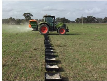
Factory settings are no substitute for spreader testing in the field. Individual spreaders, operator know how, physical properties of different products and spreading conditions have a significant impact on the even distribution of fertiliser.
